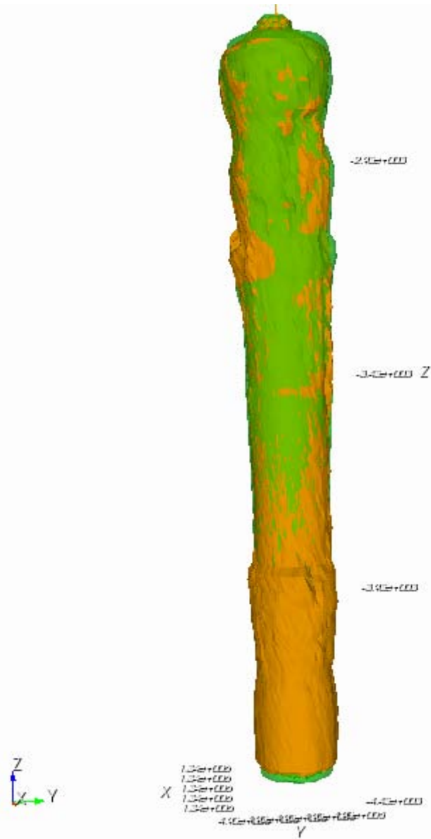
Figure 57. Superimposed sonar measurements of Cavern 101, from 1/16/2001 (green) and 9/26/2006 (yellow).
