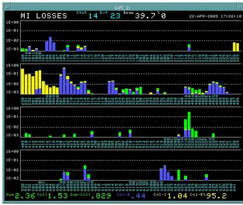
Figure 4: Logarithmic display of losses around the Main Injector. Integrated loss at the end of the cycle are displayed in green. Losses after the uncaptured beam loss overlay this in yellow. Losses at the end of injection overlay this in blue. Various sums and intensities are displayed at the top and bottom. For this display, the collimation region includes 229 - 309.
