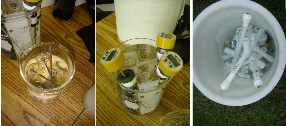
Figure D.23. Pipe system and in-line instruments are cleaned with acid solution, the left figure shows inner parts of flowrate meter is being acid washed with pH 2 solutions. Middle figure shows the cleaning of thermometer and shell of flowrate meter with pH 3 solution. Right figure shows that the pipe system, parts of solenoid valves, nozzles, and parts of totalizers were immersed into diluted vinegar solution.
