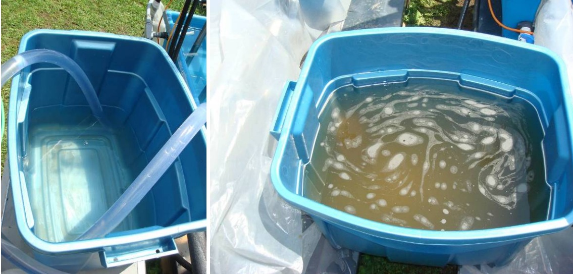
Figure D.21. Ten gallon side recirculating system was used to clean the copper coil. One gallon of vinegar was diluted to roughly 10 gallons with tap water. After 30 to 60 minutes of recirculating time. The acid wash procedure could remove the scaling. The water turned to dark brown after the procedure.
