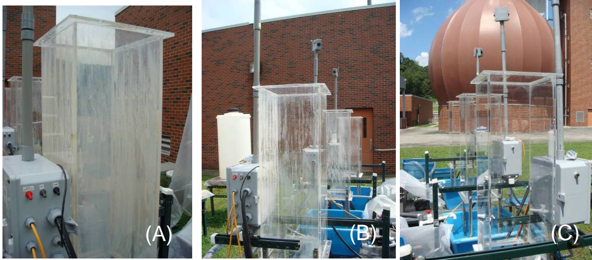
Figure D.20. From left to right, figures are showing the cleaning procedure on August 5th , including: 1. Air dried for one hour after operation stopped; 2. Cleaned by using brush and tap water; 3. Cleaned by using brush, tap water, and 4% vinegar.
