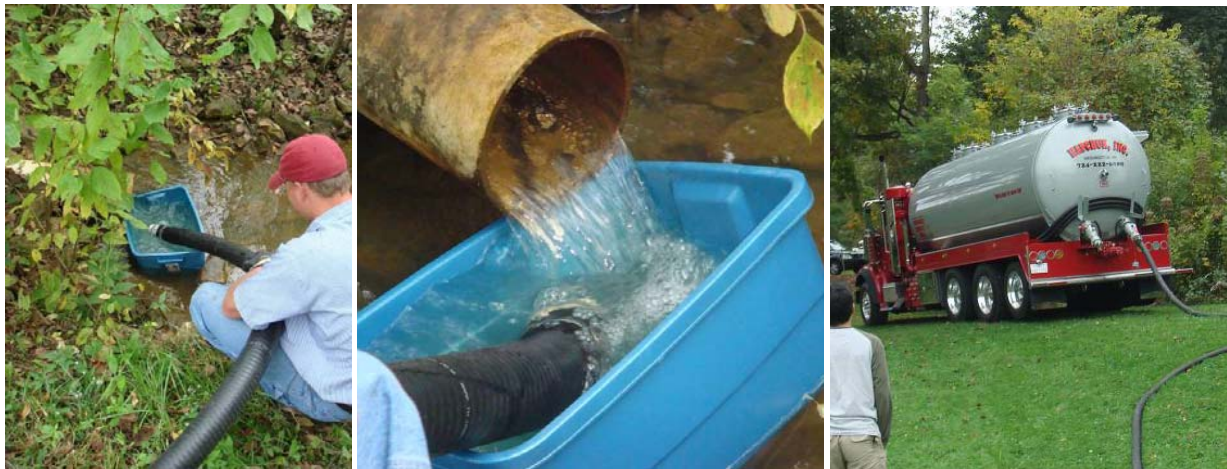
Figure E.14. Collecting treated AMD effluent at St. Vincent College constructed wetlands. The outflow rate of AMD from the conduit was 1 gal/s. The 10-gal blue container was used to prevent sediments and debris from the bottom of the stream from entering the pipe.
