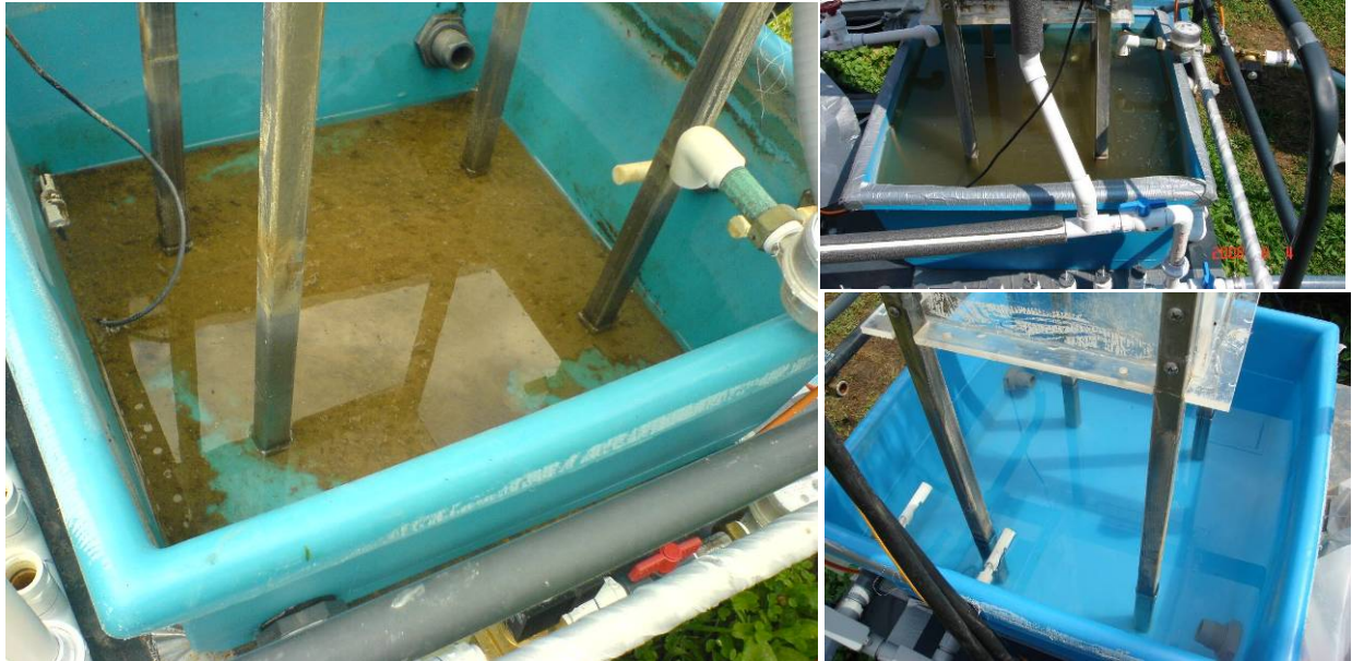
Figure D.22. Basin was simply cleaned by using brush and tap water and waste water was drained by siphon tube; small amount vinegar was used to remove solid precipitation on stainless steel legs.
