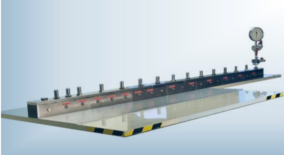
Figure 1. Photograph of the tunnel model. The charges are mounted near to the closed tunnel entrance (left end of the tunnel). The side-wall shows a number of boreholes where piezo-electric gages or the conductivity probe can be installed. The chimney-like elements on the roof can hold photo-diodes.
