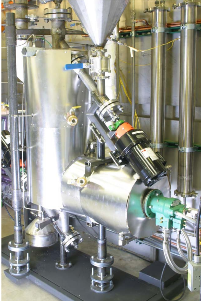
Figure 47. EERC indirectly heated bench-scale gasifier.
