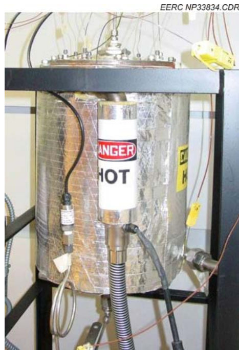
Figure 2. Catacel Corporation's novel fixed-bed FT reactor capable of operating at pressures in the range of 100–150 psig.
