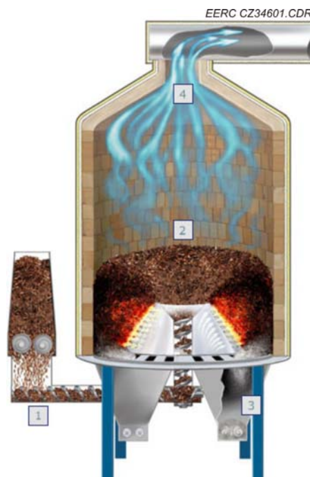
Figure 44. Image of Nexterra gasifier (31).
