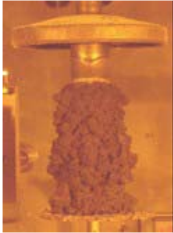
Fig. 6. Zirconium-rich cathode with uranium.
