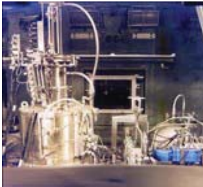
Fig. 2. Hot Cell Injection Casting Furnace
