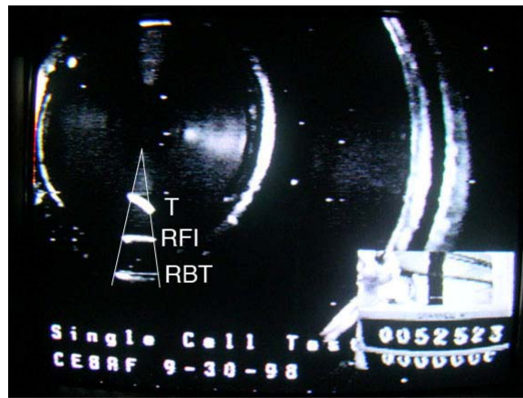
Figure 28. Track segment with a double reflection in Frame 52523. The track segment T is moving from right to left. RFI indicates the reflection in the far iris, and RBT indicates the reflection in the beam tube.
