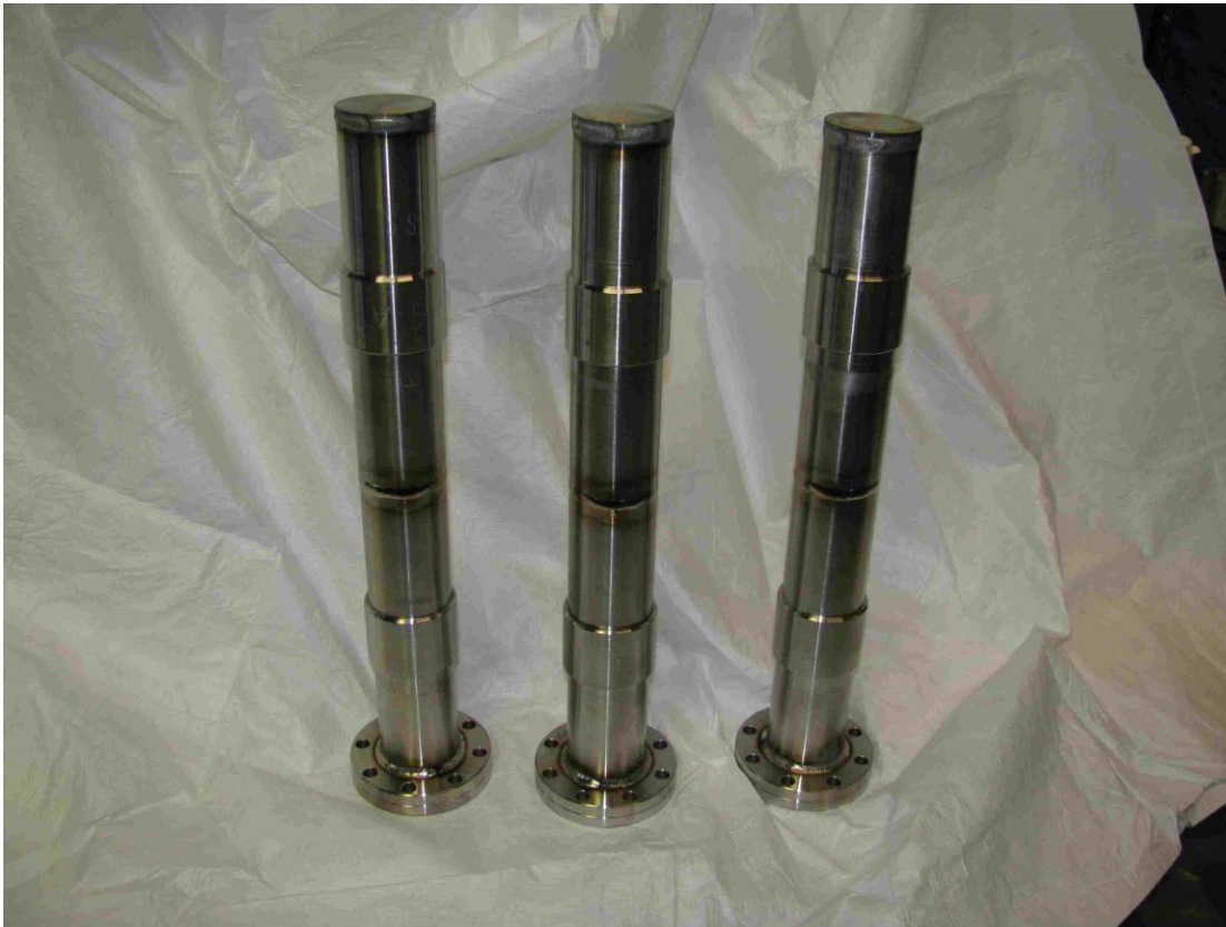
FIGURE 2. The Transition Joint Test Assemblies, 47 mm OD version. Each has a pair of transition joints.
