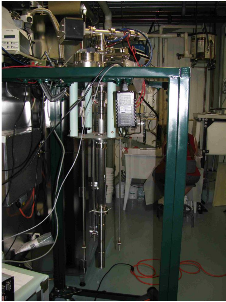
FIGURE 3. Transition Joint Test Assembly, prior to installation into the A0 Vertical Test Dewar.
