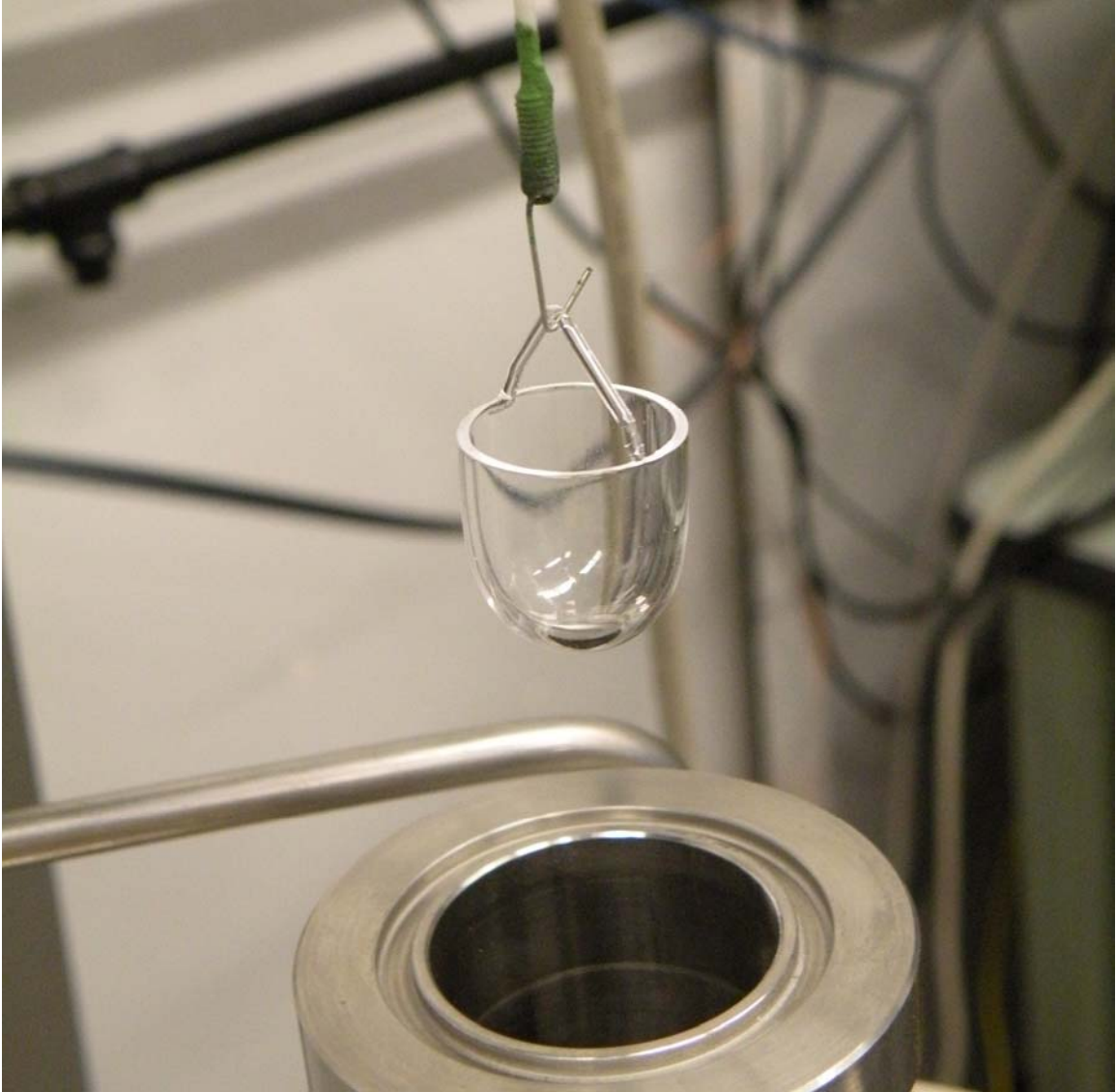
Figure 15. The all-quartz sample holder (bucket)
