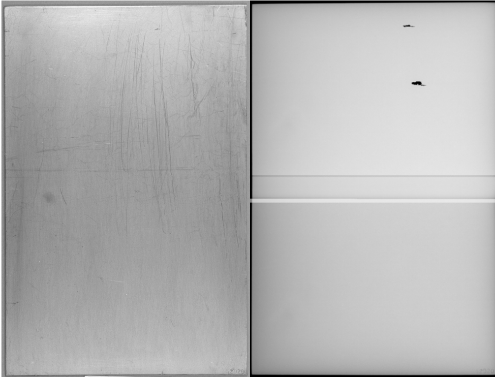
FIGURE 2. Type 301 SS annealed (front of 52D20). Cleaned specimen (left) and X-ray (right).
