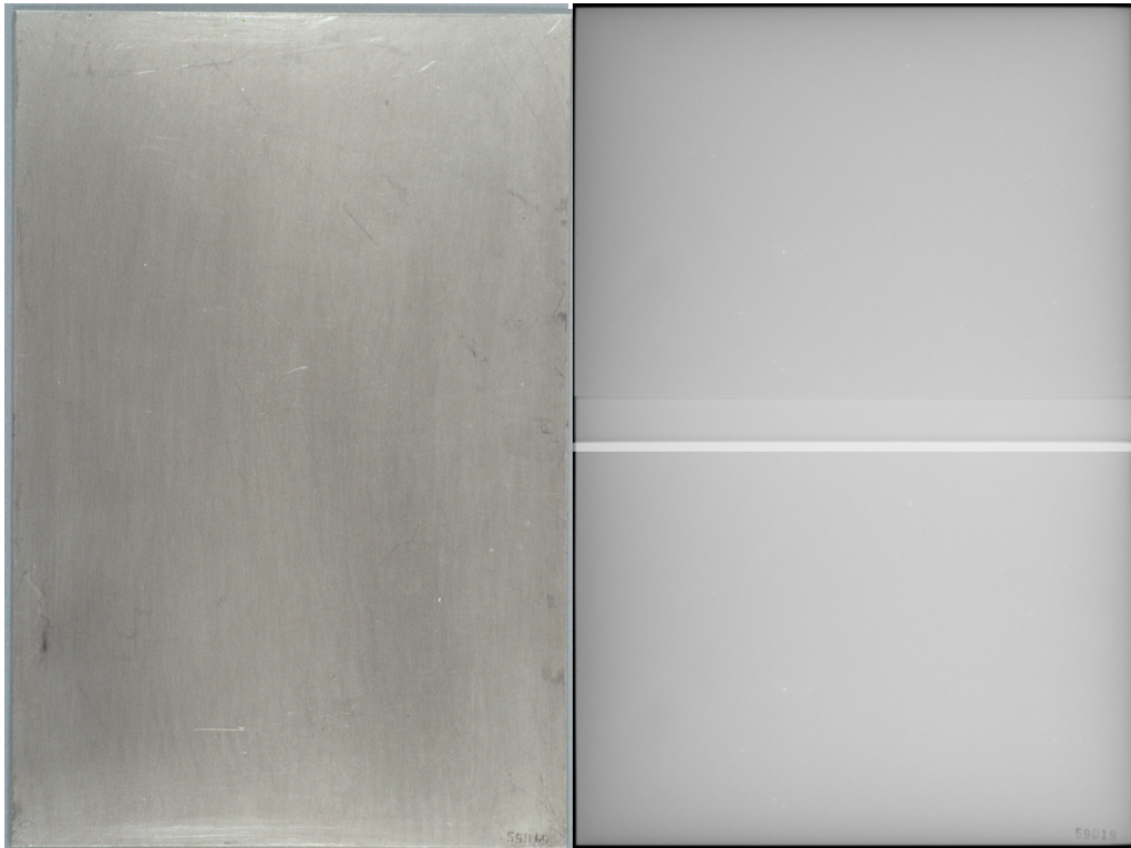
FIGURE 23. Type 316 SS sensitized (front of 59D19). Cleaned specimen (left) and X-ray (right).
