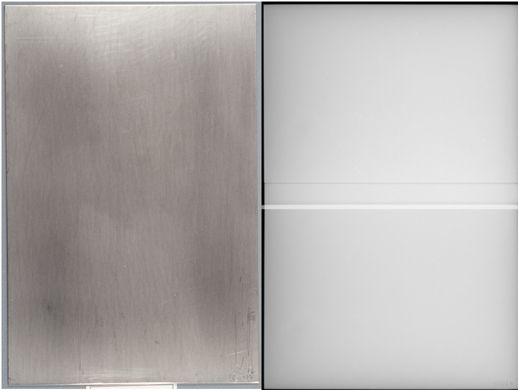
FIGURE 21. Type 316 SS annealed (front of 58D19). Cleaned specimen (left) and X-ray (right).
