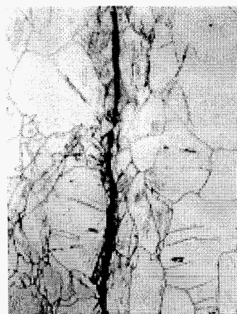
Fig. 4. Grains at the weld interface in a "bad" weld.
