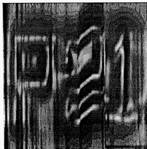
Fig. 5. Magnetic field data collected with SAMi for an etched Cu plate
