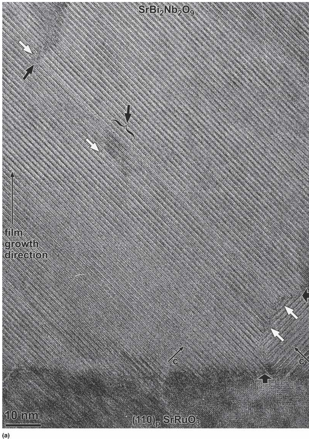
FIG. 28. The interaction of OPB nucleation mechanisms can lead to complicated defect structures. In the HRTEM image in (a), and the schematic illustration of (a) in (d), a large growth twin has overgrown a differently oriented growth twin in the early stages of film growth, providing a (001) perovskite surface. Broad arrows indicate the growth twin boundary at the bottom right of the image. In this case, the misfit has resulted in the generation of a pair of closely correlated c stacking faults, indicated by white arrows oriented parallel to the plane of the stacking fault. Near the center of the image, one stacking fault jogs along an OPB to combine with the other stacking fault, indicated by the black brace and arrow, creating a single, larger stacking fault. Soon after, on the top left, the large combined stacking fault jogs to form an OPB, indicated by the black arrow which continues through the full thickness of the film. Enlarged views of the arrowed regions are shown in (b), (c), and Fig. 24(c), respectively, (d) is a schematic of the entire defect structure in (a).
