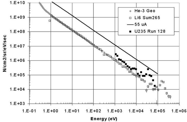
Figure 1. Surface current for FP14 at the Lujan Center, measured at  $55 \mu\text{A}$  proton current. The predicted surface current is shown as the solid line.
