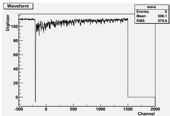
Figure 3. Typical waveform from a completed Ba<sub>2</sub> crystal assembly using a DC-720 1 GHz digitizer. One channel corresponds to 1 ns. The fast and slow components are easily recognized.
