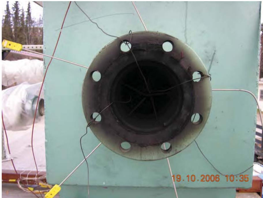
Figure 2.21. Thermocouples on the outlet of the heat exchanger.
