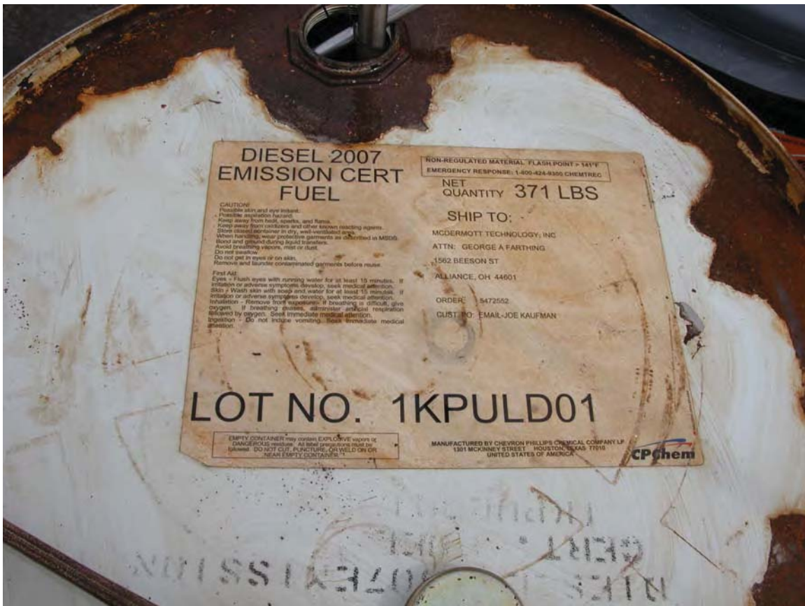
Figure 4 Low Sulfur diesel label for fuel used at INEEL demonstration. Maximum sulfur content of 15PPM.
