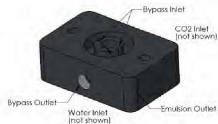
Figure 9. Schematic of microemulsion injector
