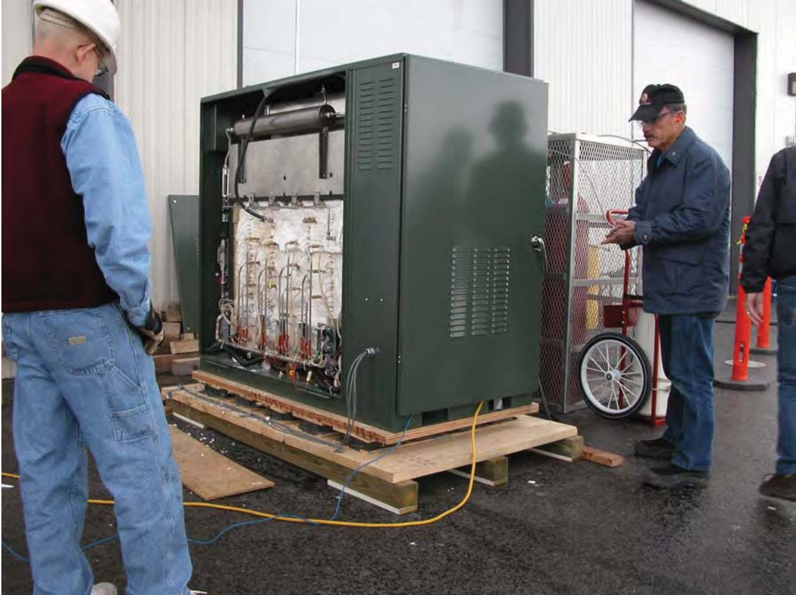
Figure 2 Acumentrics Fuel Cell at INEEL, October, 2004. Energy Alternatives Jim Buckley is standing next to fuel cell unit.
