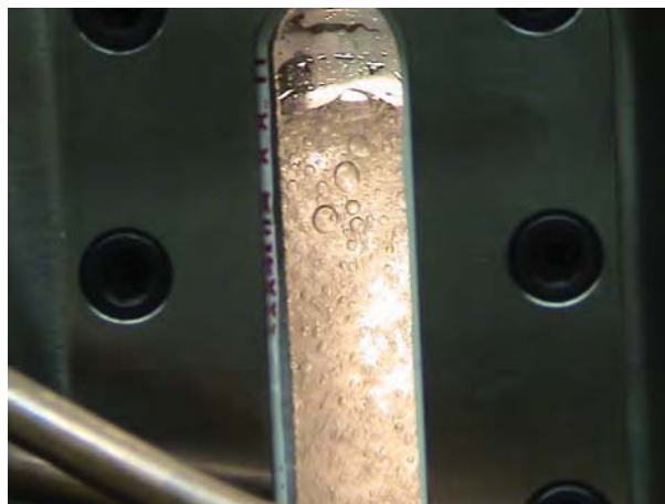
Figure 7. View through quartz window into magnetically stirred pressure cell containing liquid CO 2 and water at 15°C and 1000 psig
