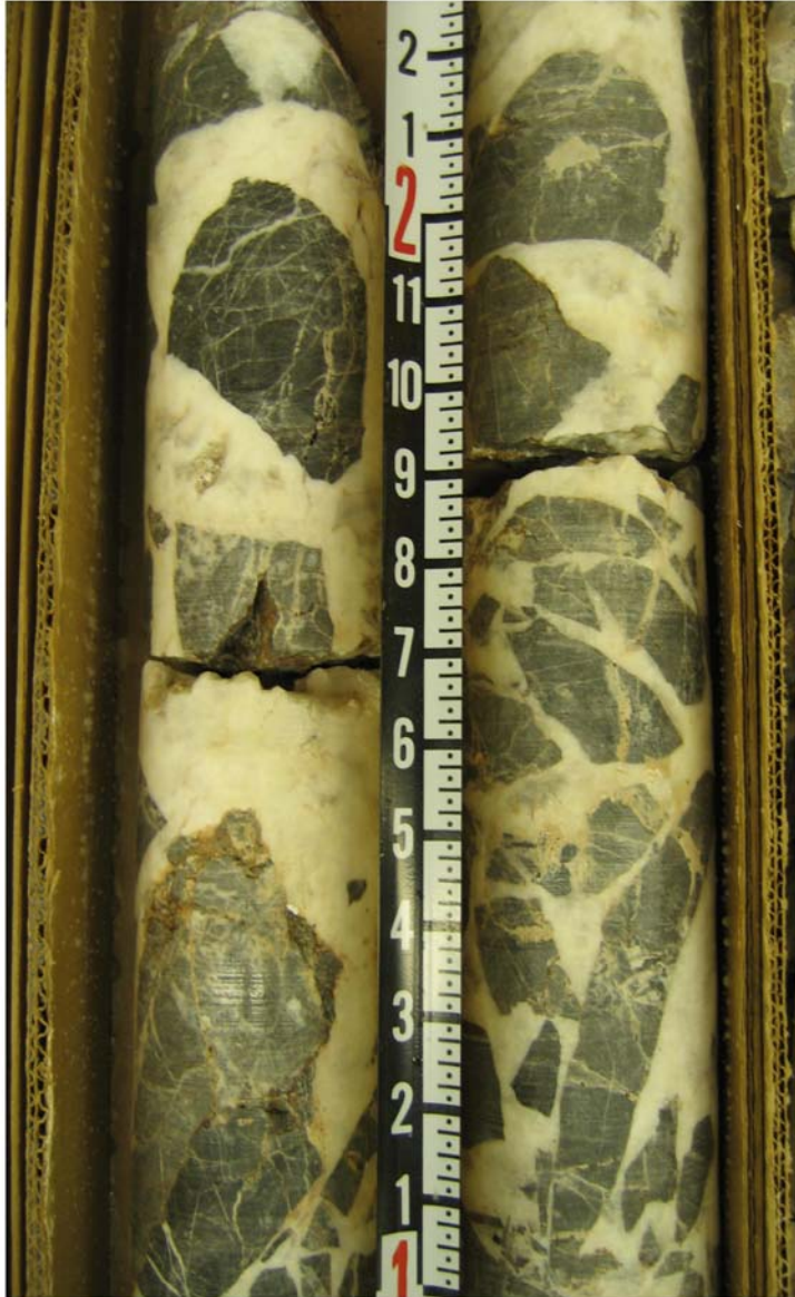
Breccia consisting of dolomite clasts within a coarsely crystalline calcite matrix. Tape measure is marked in inches.
