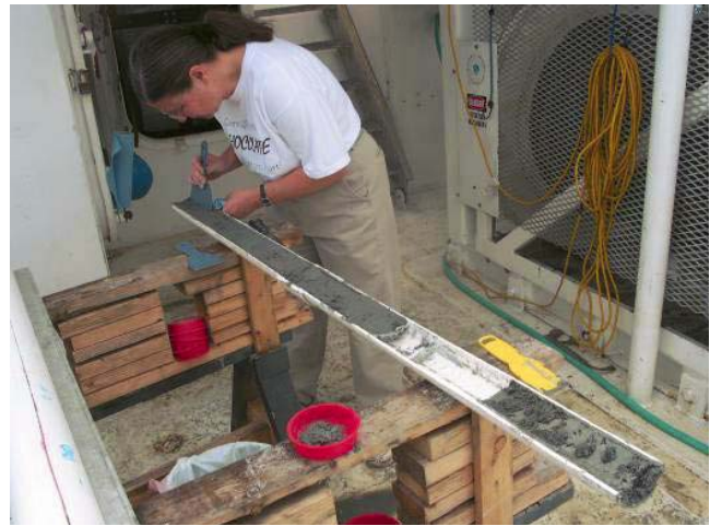
Figures 5 and 6. Section of sediment core with evidence of possible gas hydrate dissociation (left) and split core with section of gas expansion (right).
