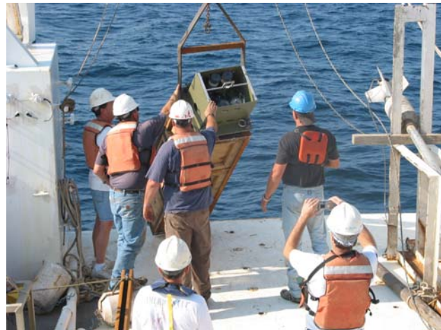
Figures 7 and 8. Recoverable osmo-pumps and sample storage units (left) and deployment of the Pore Fluid Array (right).
