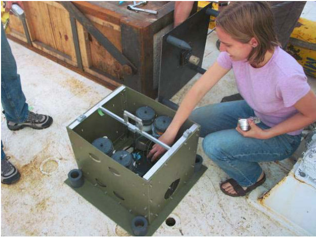
Figures 7 and 8. Recoverable osmo-pumps and sample storage units (left) and deployment of the Pore Fluid Array (right).
