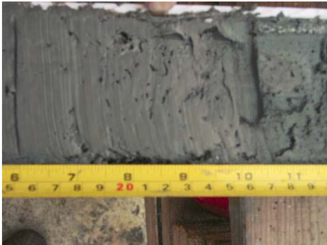
Figures 5 and 6. Section of sediment core with evidence of possible gas hydrate dissociation (left) and split core with section of gas expansion (right).
