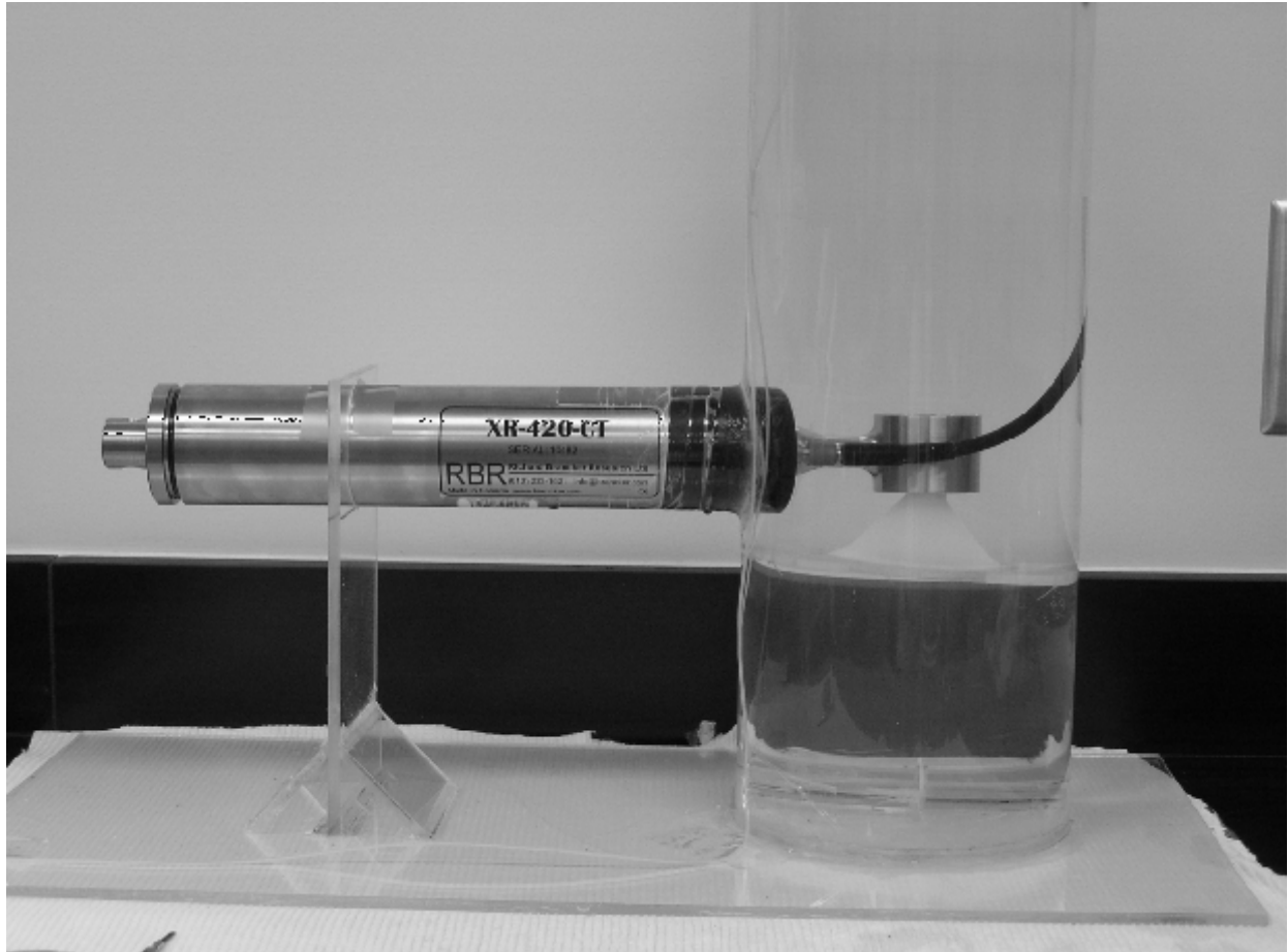
Figure 3. Laboratory test tank with Brancker conductivity sensor installed.
