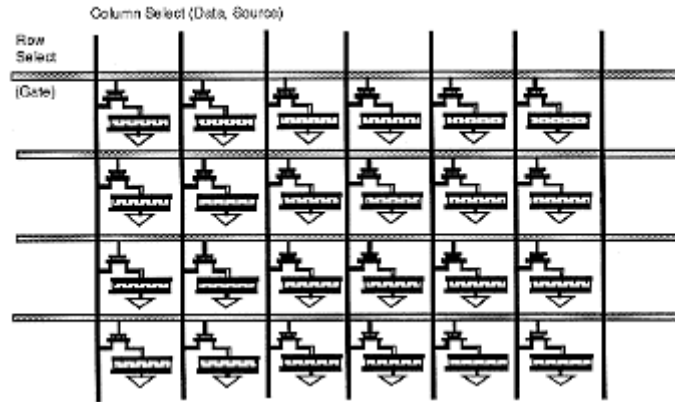
Figure 2.2. A schematic diagram showing simple TFT Active Matrix Array [11]
