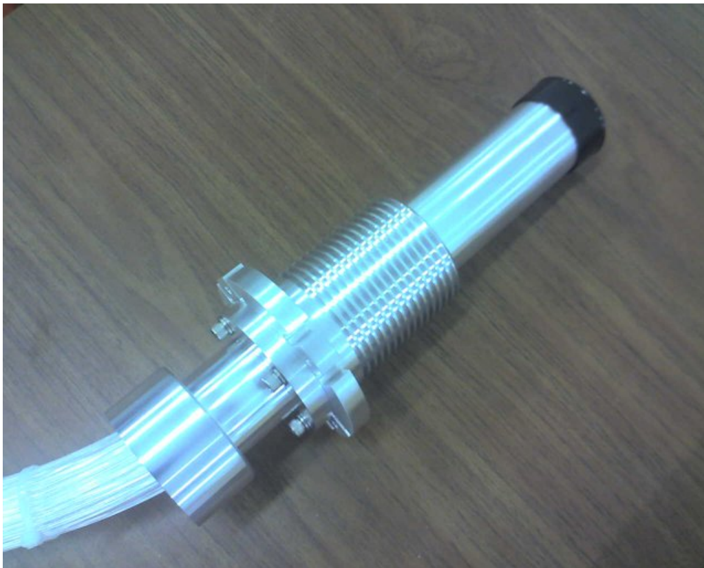
Figure 3. A picture of the newly- designed receiver. The external surface was extended to enhance the dissipation of heat.
