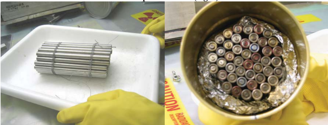
Figure 11 An array of 45 pins of MOX on the bench (left) and positioned inside a round can with aluminum foil to keep it centered (right).
