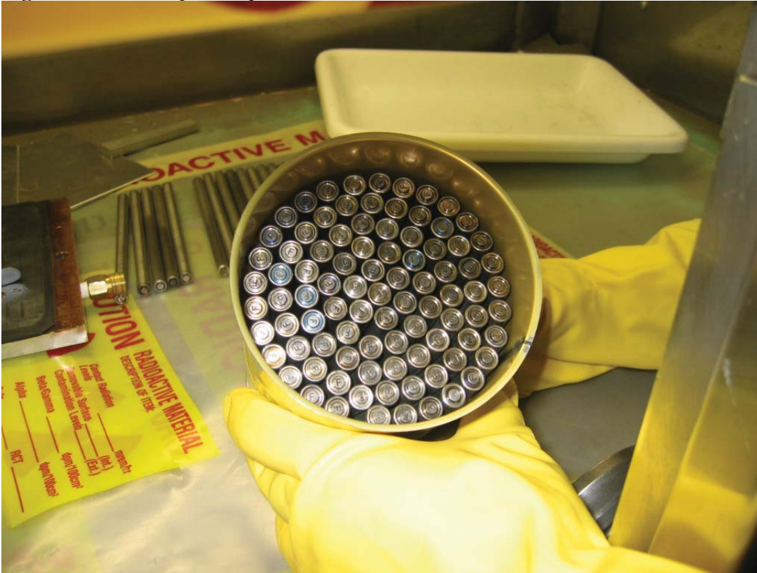
Figure 10 An array of 90 pins of MOX fuel loaded in a round can.
