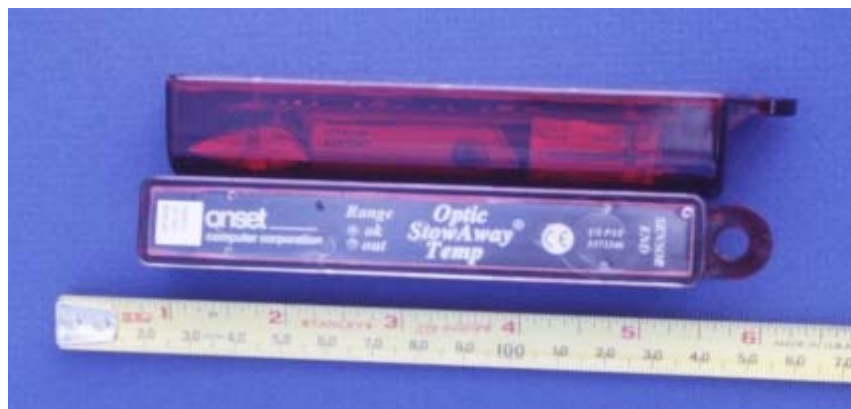
Figure A.2. Self-Contained Temperature Loggers. Loggers are approximately 12 cm in length.
