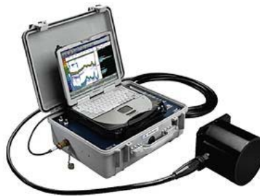
Figure F.1. DT-X Splitbeam Hydroacoustic System Used for Mobile Surveys at Grand Coulee Dam Third Powerplant in 2003
