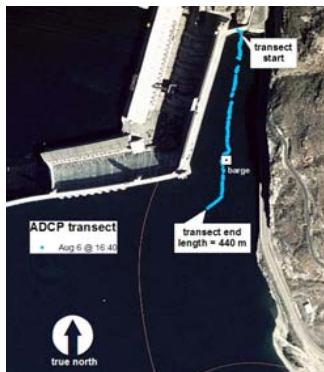
Figure D.12. Water Velocity Magnitude (top), Direction (lower) Collected on August 6, 2002, at 16:48 in the Forebay of the Third Powerplant at Grand Coulee Dam. In the plots, upstream is to the left, downstream to the right. The transect was along the centerline of the forebay (left). The directions in the lower graph are in an earth-referenced coordinate system (middle). Locations of turbine units 19 through 24 are indicated by vertical lines.
