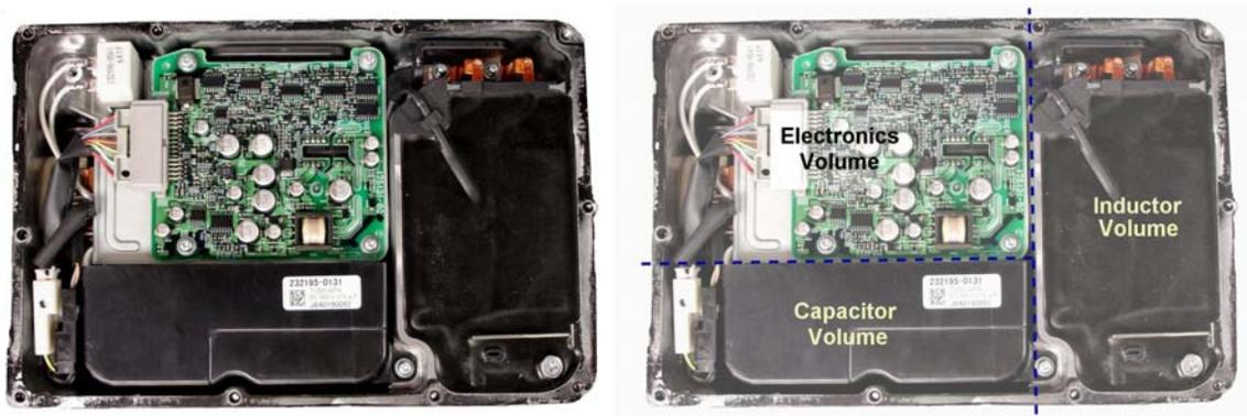
**Fig. 2.7. Converter assembly with subsections shown consistent with volume measurements.**
