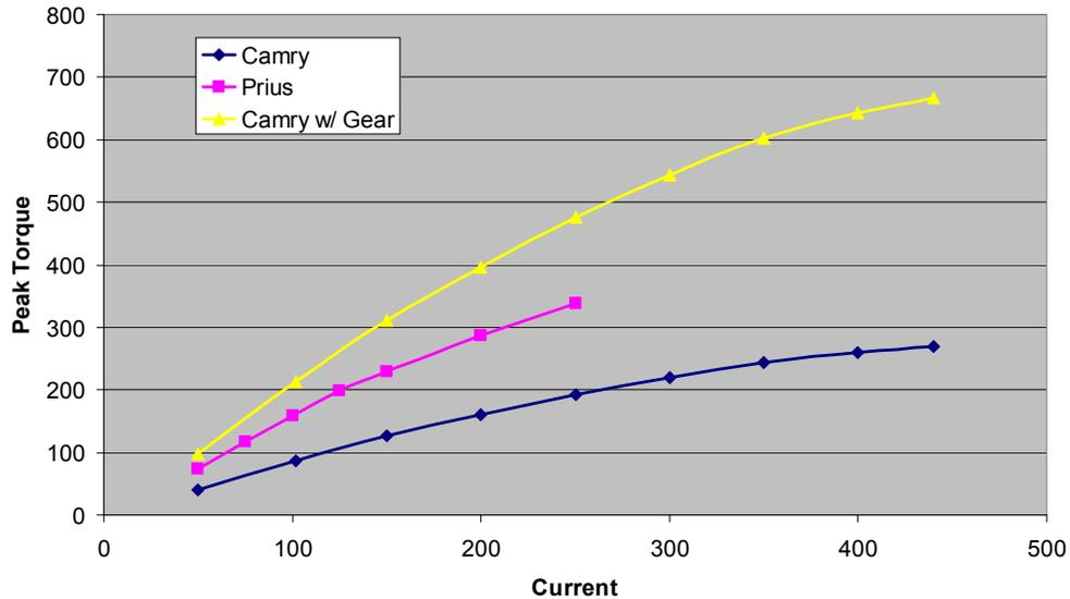
Fig. 3.15. 2007 Camry and Prius peak locked rotor torque vs. dc current.
