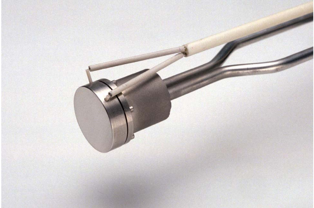
Figure 3. Sample assembly with a machined cobalt disk (2.54 cm diameter) with internal thermal couples and attached to an air-cooled chamber.
