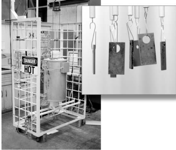
Figure 2. Cyclic oxidation apparatus for testing in atmospheric pressure steam/air mixtures.
