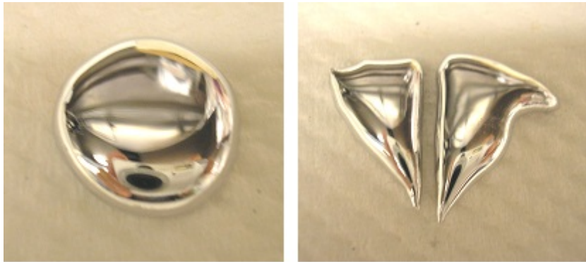
Fig. 7. Bead of pure mercury on the left assumes and maintains a roughly hemispherical shape despite probing with a plastic rod, while the same size bead of Hg – 10 wt % In on the right has its shape readily manipulated. A plastic rod was dragged through the center of each bead just prior to this photograph. Actual bead size in each case was approximately 15 mm diameter.
