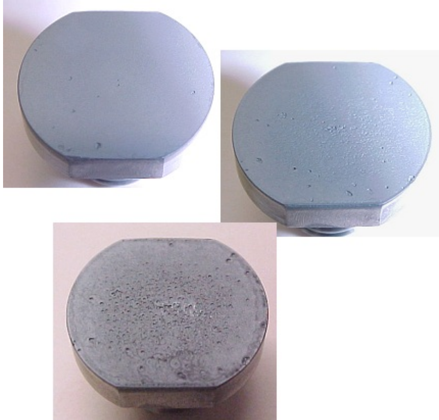
Fig. 18. Test surface of Kolsterised® specimens with a cold-worked substrate exposed to sonication in mercury for 27 h, 33 h, and 42 h, clockwise from top left. Actual specimen diameter for all buttons was 16 mm.
