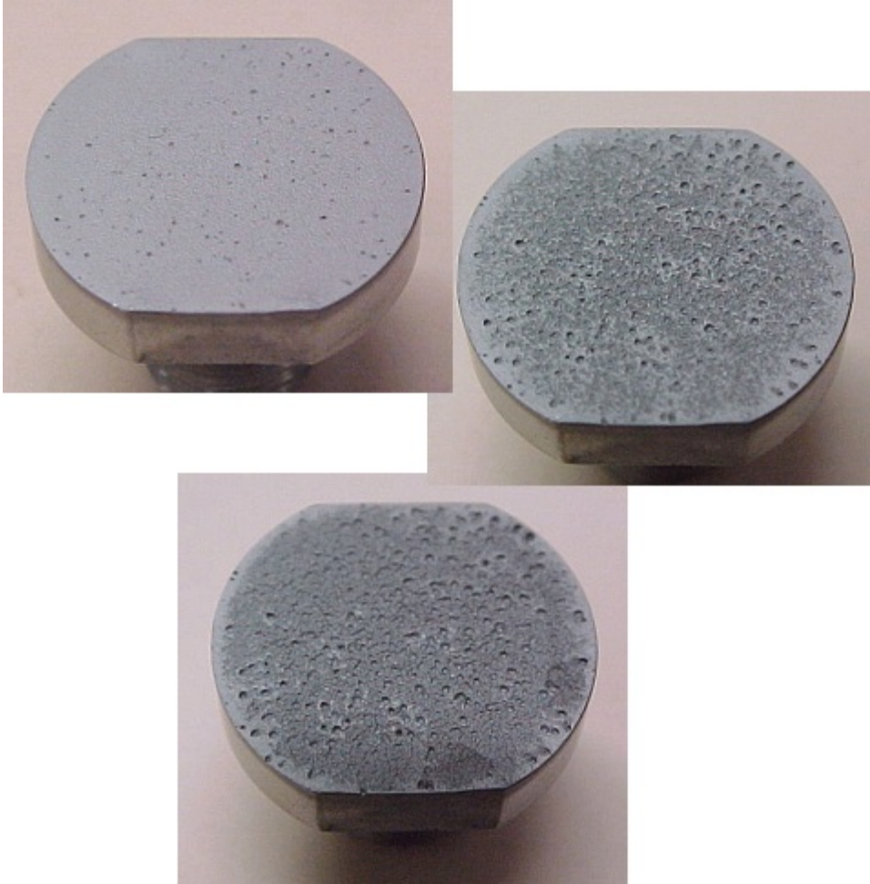
Fig. 15. Annealed-plus-Kolsterised® specimen “c” following 24-, 36-, and 42-h of sonication in mercury, respectively, clockwise from top left. Actual test surface diameter is 16 mm.
