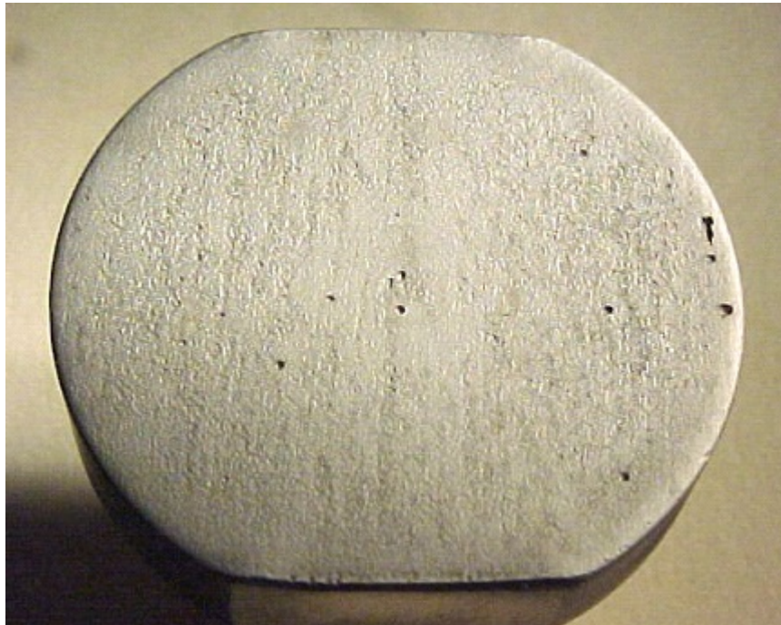
Fig. 5. Test face of specimen “a” (annealed 316LN specimen) following Kolsterising® and 20 h sonication in mercury. Actual specimen diameter is 16 mm.
