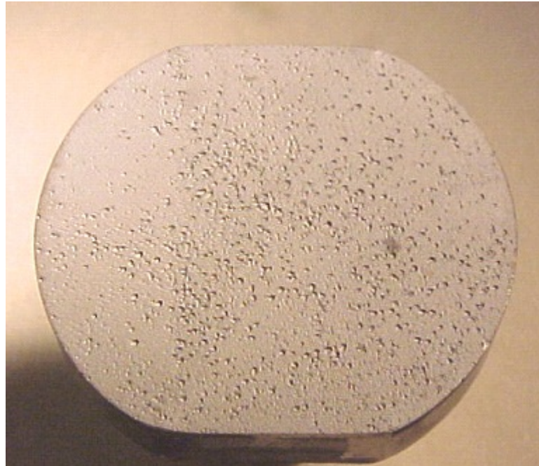
Fig. 21. As-received/untreated CW12MW specimen (actual diameter = 16 mm) following sonication for 6 h (2 mm depth) in mercury. Surface reveals non-uniform pitting damage.
