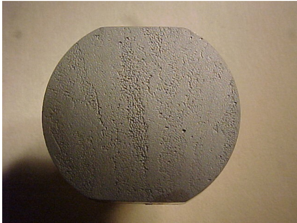
Fig. 2. Test surface of an untreated CF8M test button (actual diameter = 16 mm) following 6 h sonication (2 mm depth) in mercury. Surface relief appears related to grain orientation.
