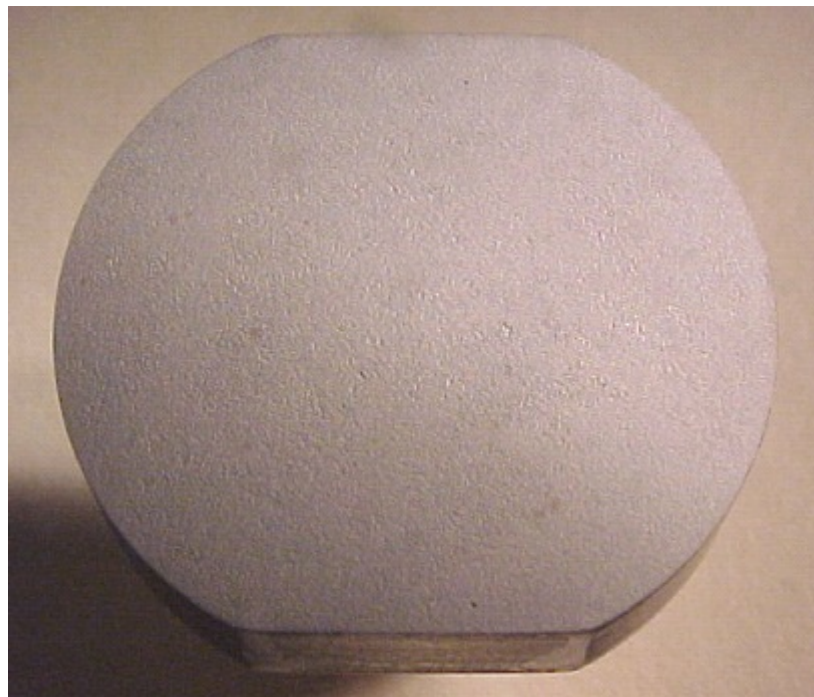
Fig. 6. As-received CD3MWCuN specimen (actual diameter = 16 mm) following sonication for 6 h (2 mm depth) in Hg. Note the relatively smooth and pit-free surface.
