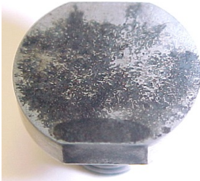
Fig. 12. Treated CA-15 specimen (actual diameter = 16 mm) following sonication for 6 h (2 mm depth) in mercury. Specimen surface reveals significant discoloration following testing.
