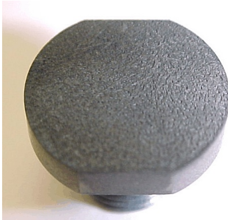
Fig. 27. As-received/untreated Class 30 gray cast iron specimen (actual diameter = 16 mm) following sonication for 3 h (2 mm depth) in mercury. Compared to other similar photos in this report, this one is at more of an angle to reveal the overlapping craters in the profile.
