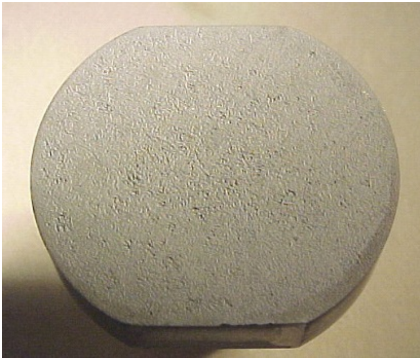
Fig. 16. As-received/untreated CD3MN specimen (actual diameter = 16 mm) following sonication for 6 h (2 mm depth) in mercury. Note the slight general roughness with no pitting.
