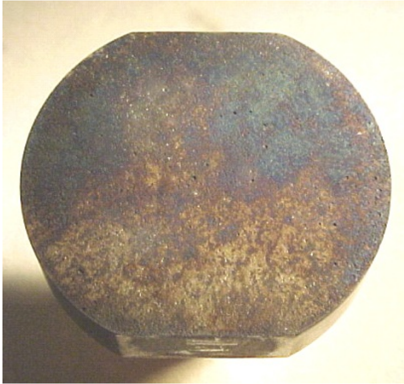
Fig. 10. As-received/untreated CA-15 specimen (actual diameter = 16 mm) following sonication for 6 h (2 mm depth) in mercury. Note significant discoloration and pits scattered across the surface.
