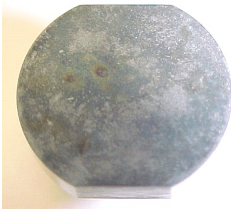
Fig. 25. As-received/untreated HC-600 specimen (actual diameter = 16 mm) following sonication for 6 h (2 mm depth) in mercury. The test surface shows a general surface roughness of \sim 15 \mu\text{m} as well as slight discoloration.
