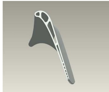
Figure 9. Solid Model of the NASA E 3 Blade, Created Using Pro/Engineer and the Finite Element Analysis Application ANSYS
