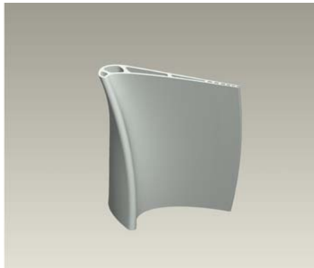
Figure 9. Solid Model of the NASA E 3 Blade, Created Using Pro/Engineer and the Finite Element Analysis Application ANSYS
