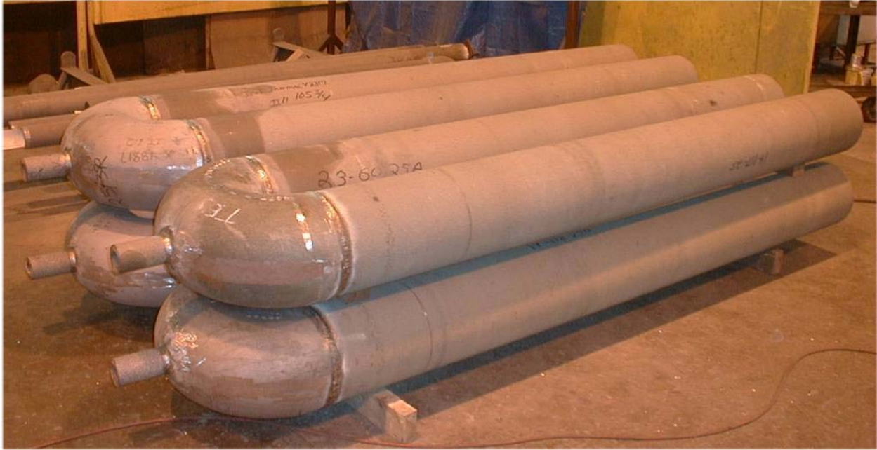
Figure 4.35: Typical radiant-tube assembly fabricated using newly developed HP alloys.
