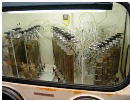
Figure 1. Columns of FRC Area 2 sediment (total U = 257 mg kg -1 = 1.08 mmol kg -1 ) in N 2 glovebox. The columns are being supplied with either lactate or acetate, at OC concentrations from 0 to 100 mM.
