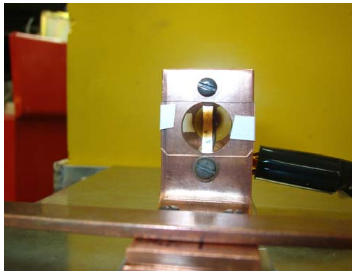
Figure 14: Irradiation target assembly with attached pieces of laboratory glass slides.
