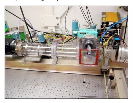
3rd generation GISAXS apparatus (SSRL beamline 1-4). Sample enclosure has door with red outline connected to He beam path. 2D detector system is at left along with beam stop and photodiode beam detector. Sample is aligned both vertically and to the proper grazing-incidence angles with computer controlled stepper drives. He path can be extended at will by adding other sections.
