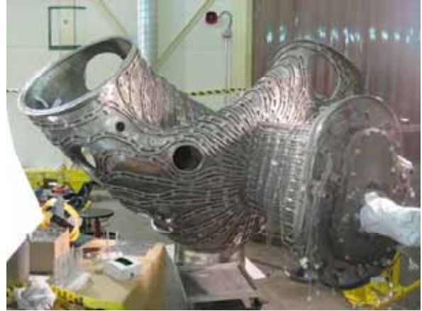
Fig. 7. Vacuum vessel sector with installed service.
