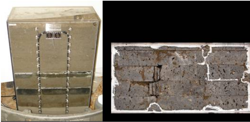
Figure 4. Layered sandbox instrumented with ERT electrodes to monitor water, tracer, and polymer movement in 3D.
