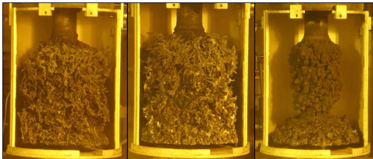
Fig. 3. Three cathodes produced during the second ER batch of the integrated efficiency test.
