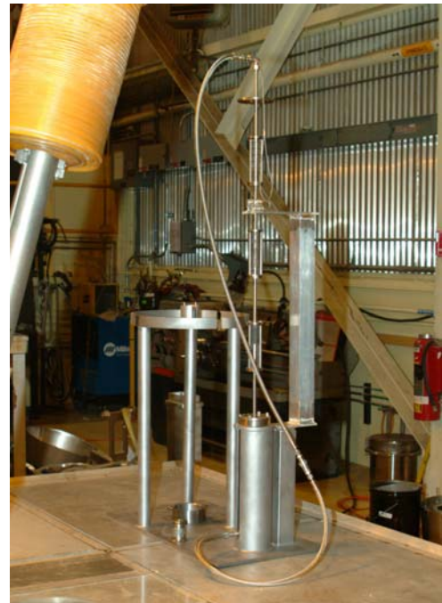
Figure 10 DEOX OTS loading/unloading equipment
