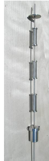
Figure 4 DEOX Off-Gas Trapping System
