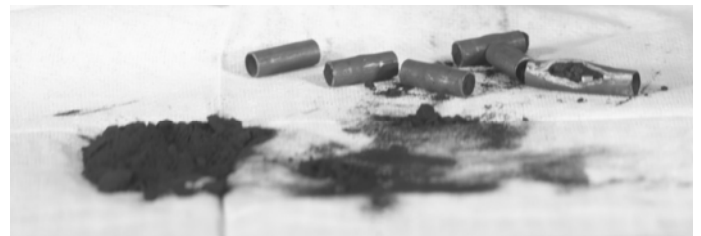
Figure 1 Spent fuel after voloxidation experiment
