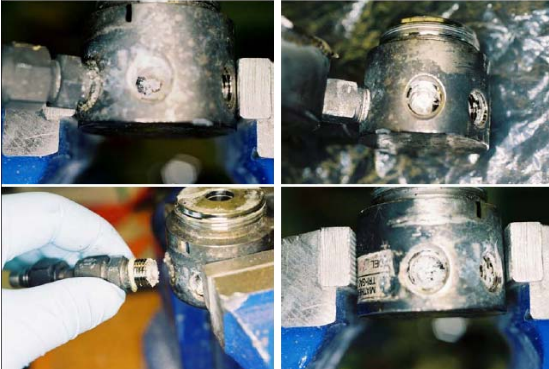
Figure 4. AEC's PCV-23, showing ports after the accident.
