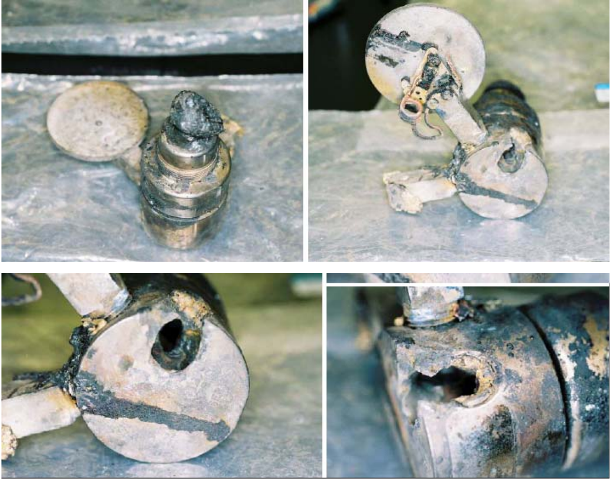
Figure 6. PCV-16 valve showing heavy combustion damage at the outlet port (shown lower).
