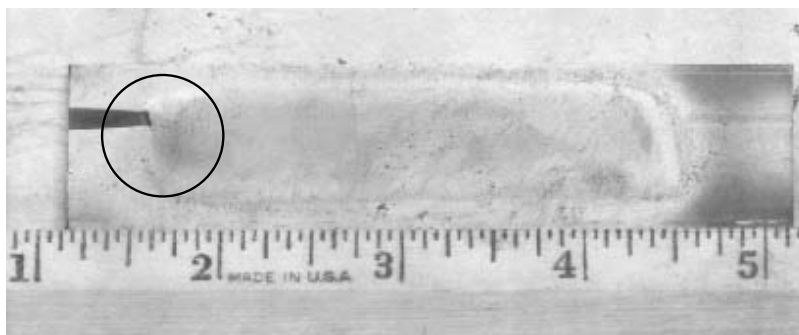
Figure 10. Breached mini-plate from RERTR-5 experiment.
