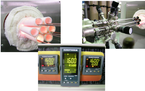
Fig. 19. Steps taken to reduce calibration costs (including use of multiple process tubes with inert gas flow control and implementation of programmable furnace control).
