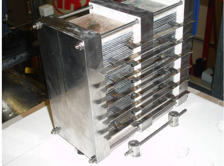
Figure 8. One-half of ILS module showing electrical interconnections.
