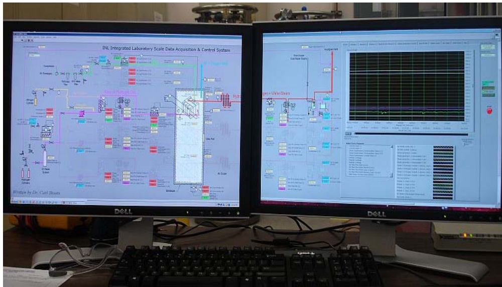
Figure 18. Screen display of the INL-developed data acquisition and control program. This program was written using the National Instruments LabView software.
