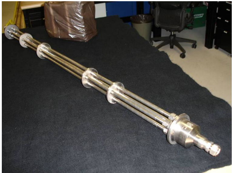
Figure 15. Air heater and steam superheater internal piping.
