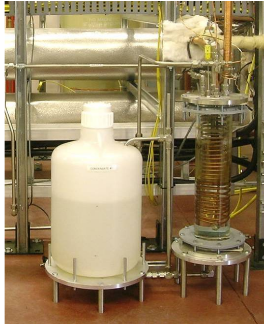
Figure 16. Condenser and condensate tank.
