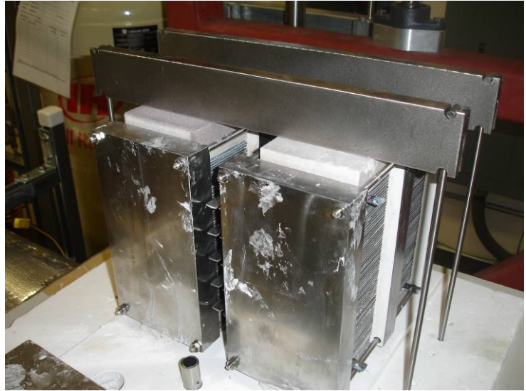
Figure 10. ILS module with spring-loaded compression bars.
