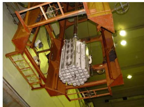
Figure 13. Loaded VPVR/M cask basket being transferred into the Building 101A hot shop/pool area.
