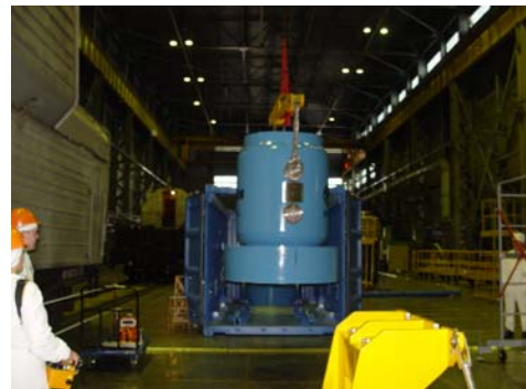
Figure 12. Cask unloading from the International Shipping Organization container in Building 855.
