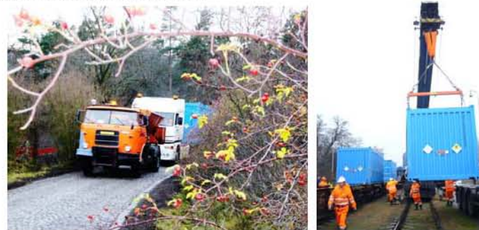
Figure 16. Photographs showing a loaded tractor trailer being pulled out of the High-Level Waste Storage Facility area and a loaded International Shipping Organization container being transferred from truck to railcar.
