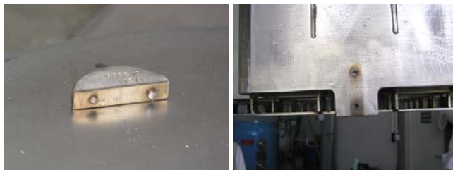
Figure 6. Photographs showing the broken spacer and the bottom of the cask basket where the spacer was attached.
