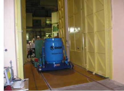
Figure 8. The VPVR/M cask being moved into the Away from Reactor storage area.
