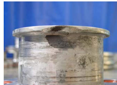
Figure 4. Cask trunnion wear, resulting from loosening of the tiedown system during transport.
