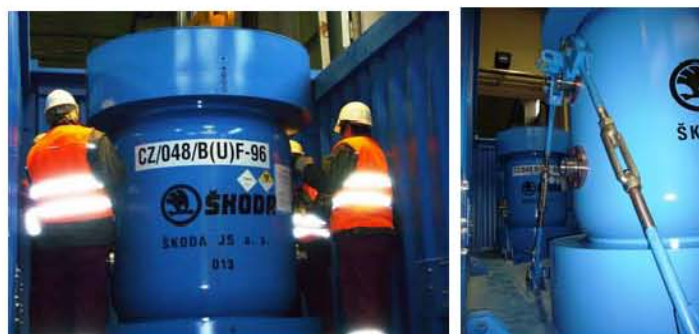
Figure 15. Photographs showing VPVR/M casks being loaded into an ISO container and tied down.
