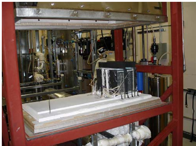
Fig. 2. Hot zone enclosure with one module installed.
