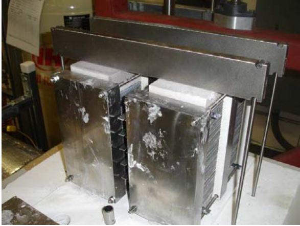
Fig. 7. ILS module with spring-loaded compression bars.
