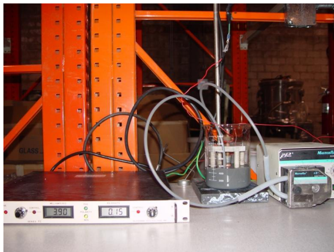
Figure 12: Electrophoretic deposition setup to deposit SiC.
