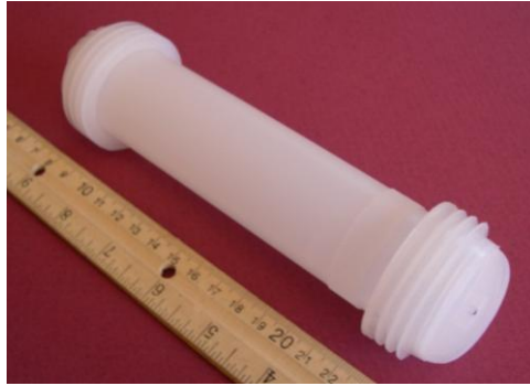
Figure 21: Polyethylene vessel (rabbit) used to place the samples in the irradiation chamber.
