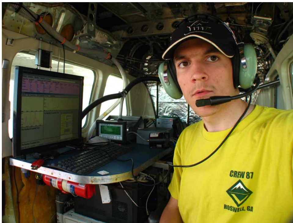
Figure 5. Interior cabin of the Skymaster showing the data logger (left), DataRam 4 PM-10 sampler (center), and split sampling line to vacuum booster pump and DataRam 4 (see subsequent description).
