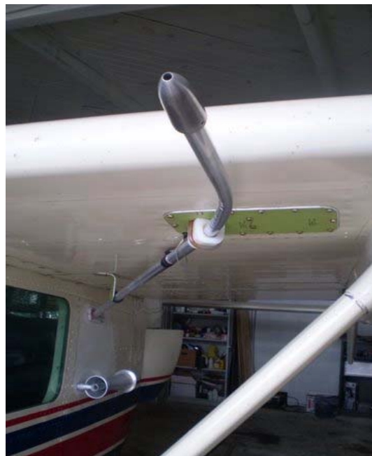
Figure 8. Isokinetic sample line inlet installed on the ARC Skymaster (for the DataRam 4).
