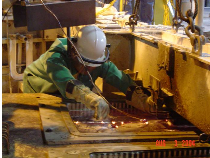
Fig. 4.1.2. A researcher placing a temperature jig into the molten aluminum in a DC casting mold at Aleris International's Newport plant.
