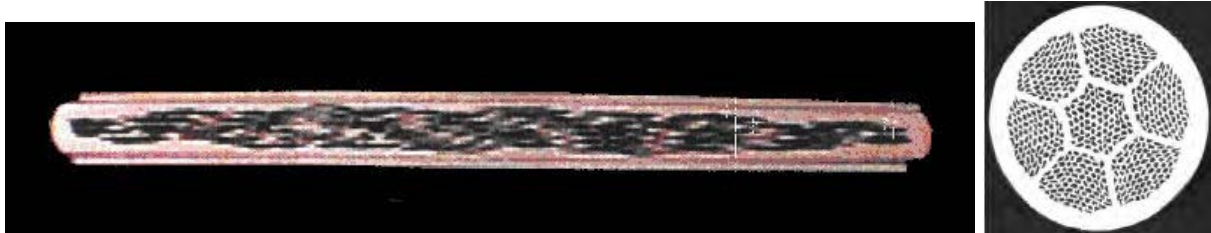
FIGURE 2. Transverse cross section of High Strength BSCCO-2223 tape showing 55 filaments of BSCCO-2223 embedded in a metal matrix of silver alloy and 37 \mu\text{m} strips of stainless steel on top and bottom of tape (left). Transverse cross section of unreacted BSCCO-2212 OST 85 \times 7 wire (right).
