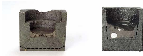
Fig. 3: Cross sections (a) a conventional 90% chrome refractory, and (b) ARC improved refractory following exposure to a coal slag at 1600°C. The depth of slag penetration is marked in each case.
