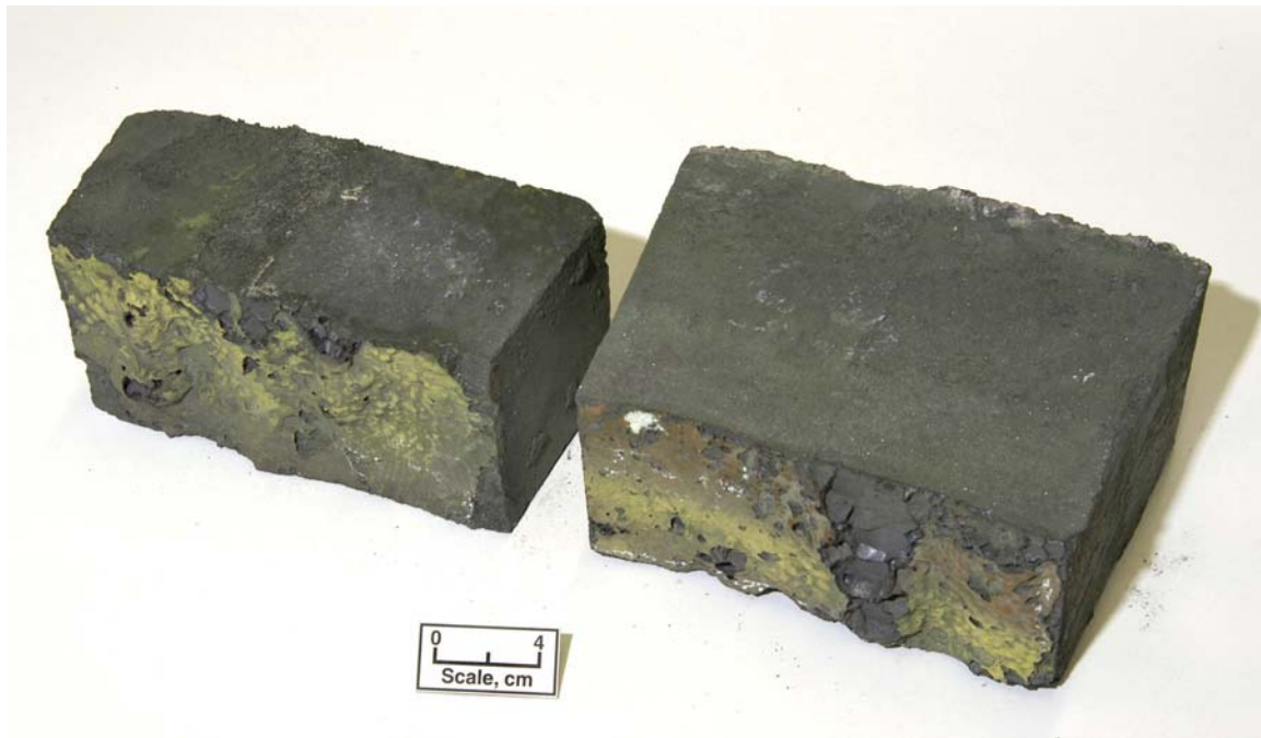
Figure 5. Refractory brick following 14-months in service in a coal-fired slagging gasifier. The NETL-developed refractory, on the right, has clearly experienced less material loss during service (original dimensions were identical in the two brick).
