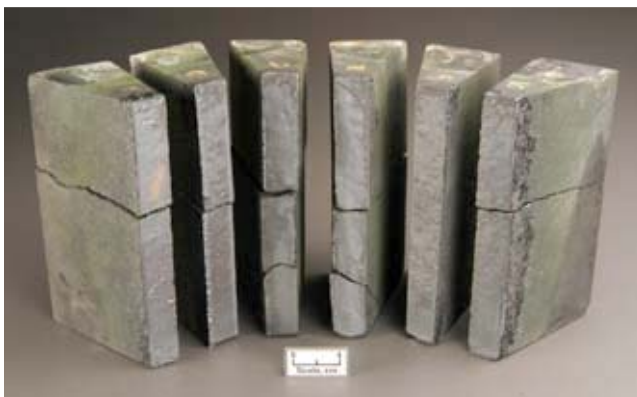
Figure 2. NETL-developed refractory (top) and commercial refractory (bottom) following exposure in the rotary slag test.
