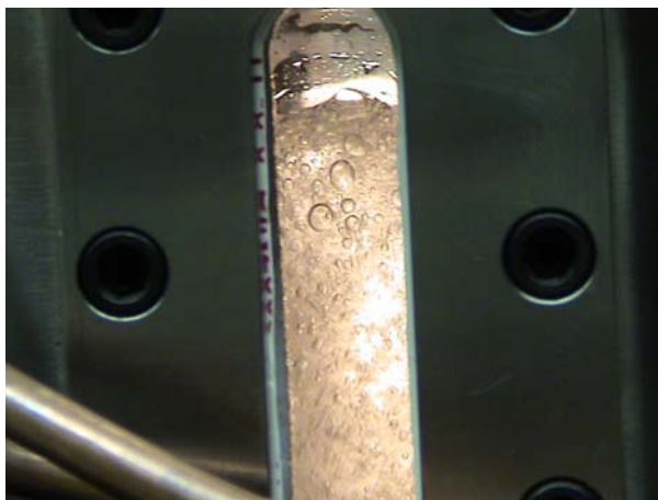
Figure 7. View through quartz window into magnetically stirred pressure cell containing liquid CO 2 and water at 15°C and 1000 psig
