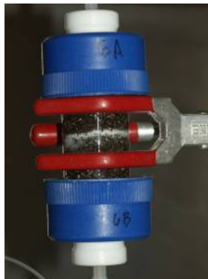
Figure 7. Photo Displaying the Apatite Barrier Placed in the Middle of a Sediment Column Composed of the <2-mm Fraction from the 300 Area
