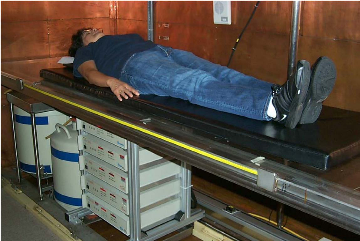
Figure 1. Counting geometry for PNNL's coaxial germanium scanning system
