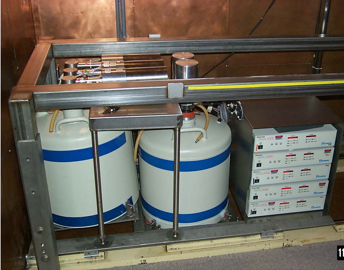
Figure 2. Five coaxial germanium detectors and electronics
