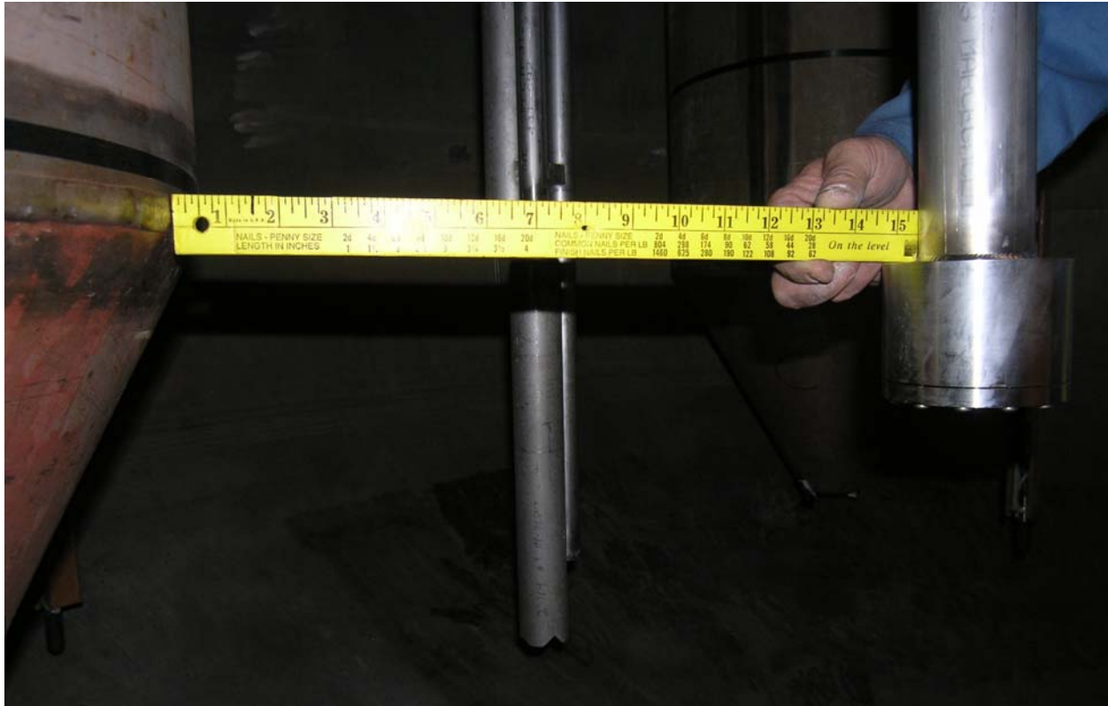
Figure 3.7. Accelerometer Housing Inside the Tank in 4-PJM Configuration (the distance from the PJM was changed slightly after this picture was taken)
