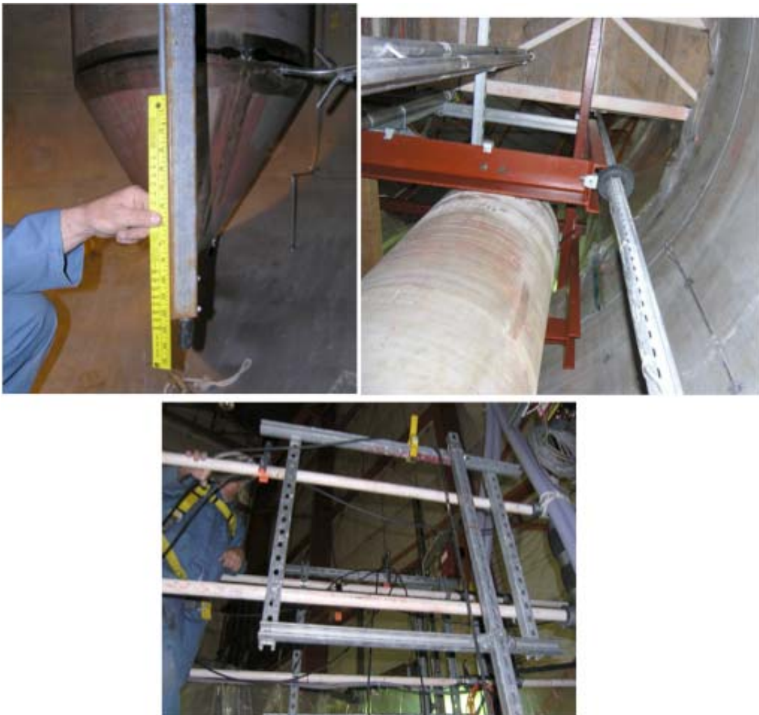
Figure 5.3. Hydrophone Mounting Columns (top left, bottom end with black tip of hydrophone protruding from the end; top right, rising shaft with rubber snubber mounted on red crossbeam; bottom, top of column attached to frame mounted on handrails above tank)
