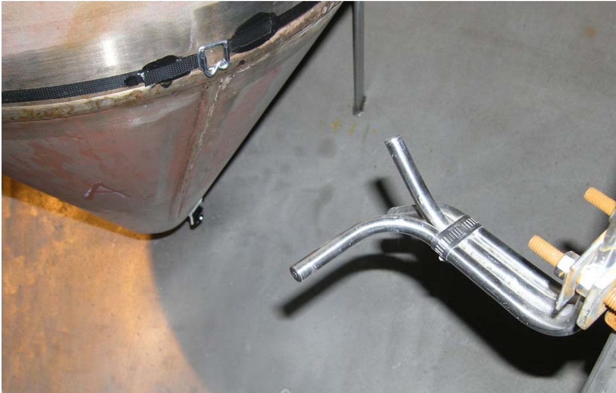
Figure 3.5. Lower In-Tank Pressure Sensors in the Tank (4-PJM configuration). Note the flush mounting of the diaphragm on the tip of the probe.
